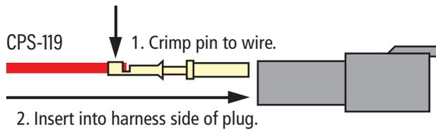
Use tool RWT-005 to crimp the pins.
