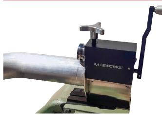
Unwind the Tri-Shaped Handle on top, insert tube between the rollers on the left hand side, and wind the tri-shaped handle back down, to hold the tube in place. Do not apply a large amount of pressure at this stage.
