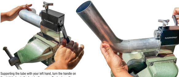
the right to begin the bead roll process. For best results, take your time and gradually apply more pressure to the tri-shaped handle on top.
