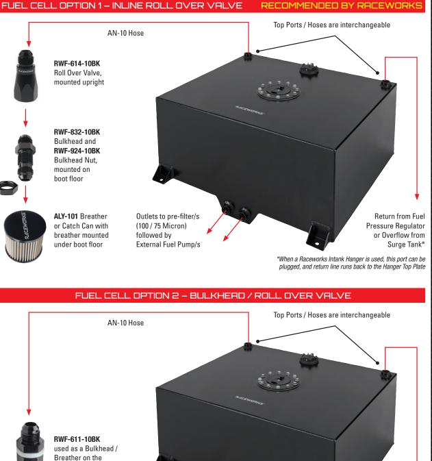
Outlets to pre-filter/s (100 / 75 Micron) followed by External Fuel Pump/s
