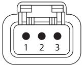
Looking into the back of the connector or sensor
