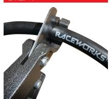
Cut hose to desired length with hose cutters, and fit hose end into vice jaws.
