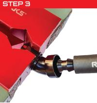
Quickly shake as much water off the hose as possible, before pushing the hose over the barb, until it seats snugly under the trim ring.
