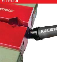
This shows the hose correctly fitted so that it sits snugly under the trim ring.
